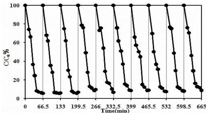
Fig. 5. Durable tests for degradation of aqueous BPA using 4.0BT (BPA=20 mg/L, pH=6, Q=3.6 cm<sup>3</sup>/min, t=66.5 min).
