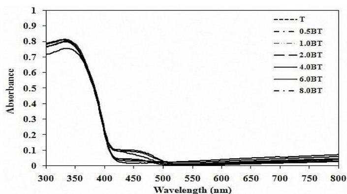
Fig. 2. UV-Vis absorption spectra of various photocatalysts.
