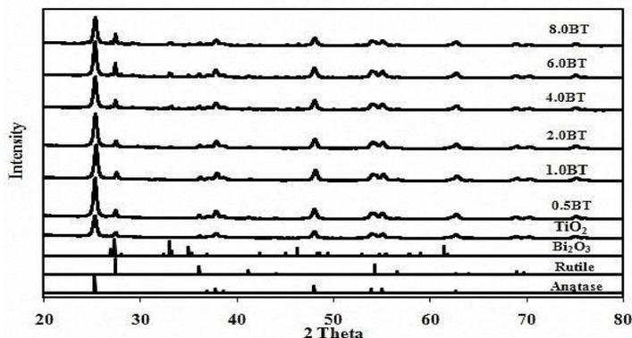
Fig. 1. XRD patterns of various photocatalysts.
