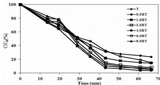
Fig. 3. BPA degradation of various photocatalysts under simulated sunlight (BPA=20 mg/L, pH=6, Q=3.6 cm<sup>3</sup>/min, t=66.5 min, λ= 250-1100 nm).
