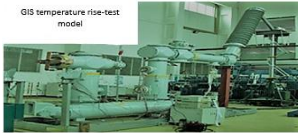
Fig. 29. GIS temperature rise-test model.
