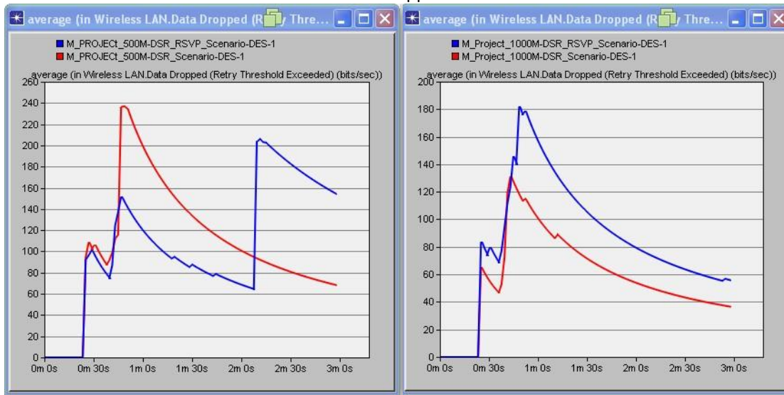
Fig. 6. Average data dropped of DSR route, Scenario 1 Fig. 7. Average data dropped of DSR route, Scenario 2.
