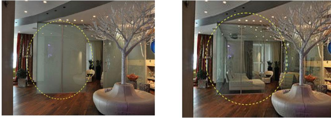
Fig.5. making use of electro-chromic smart glass as partitioning space.
