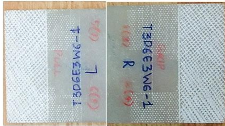
Fig. 6. Roughened end strips of specimen.
