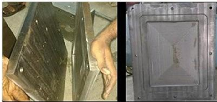
Fig. 4. Matched die mould of EN 8 steel plate.
