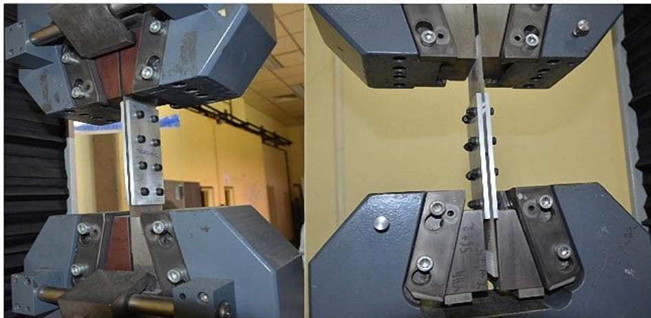
Fig. 5. Test set up on Instron universal testing machine.
