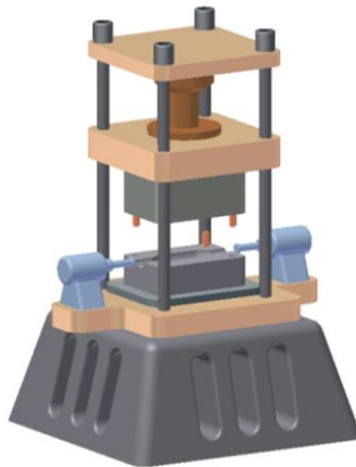
Fig. 1. Prototyped hydroforming system.
