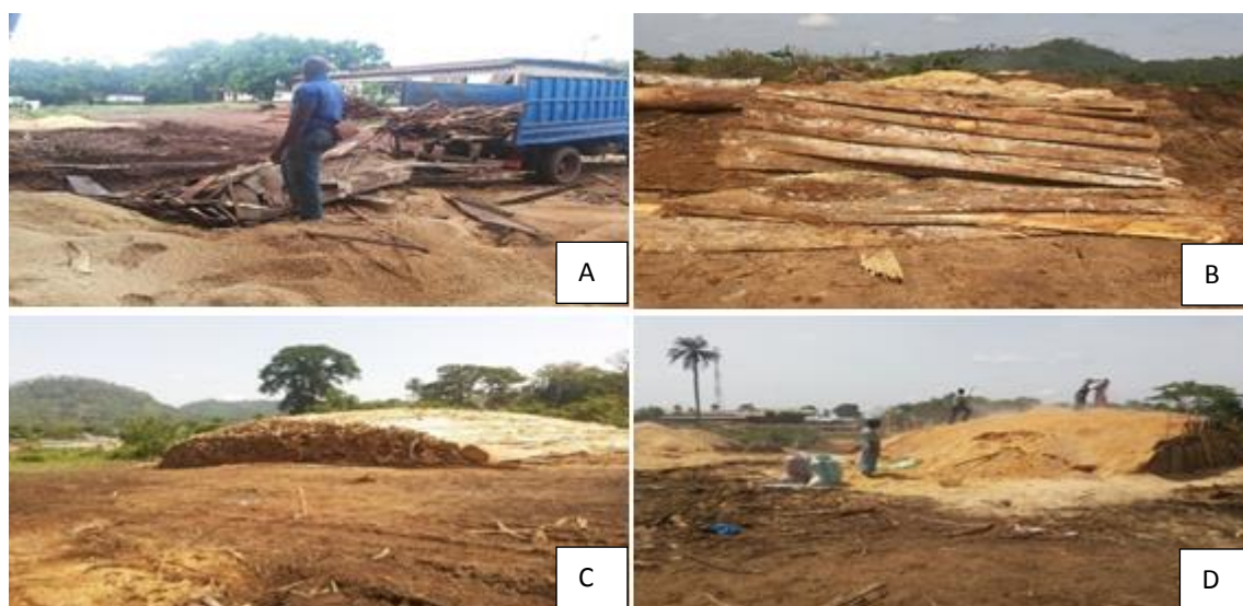
Fig. 15. Illustrations of the actions carried out in Scierie et Menuiserie du Tonkpi (SMT), A = waste removal, B = storage of slabs, C = setting up a furnace, D = furnace in operation.
