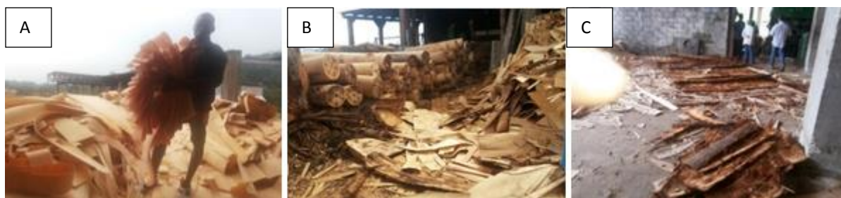
Fig. 7. Illustrations of peeling wood waste, A = unwinding slats, B = wood core and strip, C = bark.
