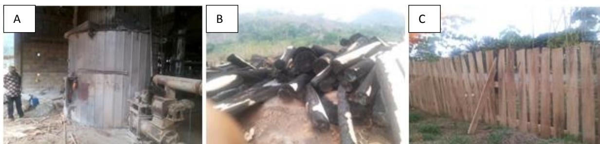
Fig. 12. Illustrations of recovery channels African Wood company's, A = boiler, B = waste burning, C = fences made with wood waste.
