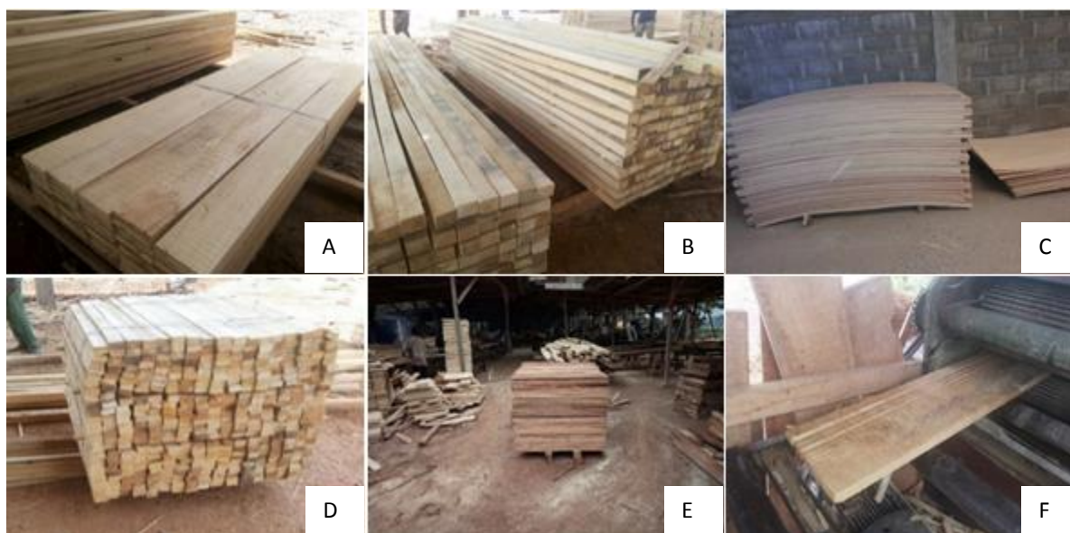
Fig. 5. Illustrations of the products obtained in timber industries, A = boards at Ets Coulibaly, B = rafters at Afr. Wood, C = plywood in Afr. Wood, D = slats at GIBT, E = pallets at SMT, F = battens at GIBT.
