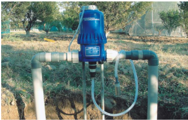
Fig. 3. Fertigation with injection pump.
