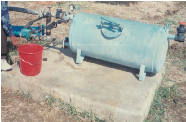
Fig. 2. Fertigation with venture.
