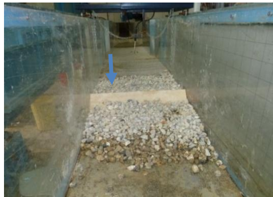
Fig. 4. downstream protection of bed.
