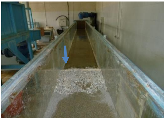
Fig. 3. upstream protection of bed.
