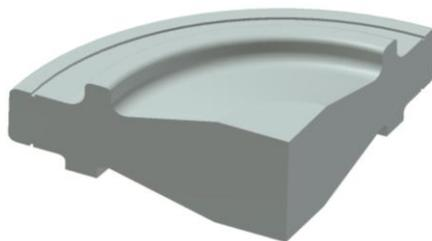
Fig. 1. Quarter portion of turbine wheel.
